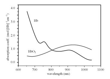
Fig. 2. Light absorption curve of  $HbO_2$  and Hb
