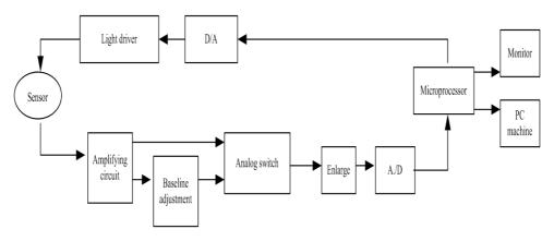
Fig. 1. Oxygen saturation detection block diagram
